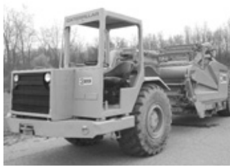
'78 Cat 613B motor scraper, 3208 Cat dsl., self-loading, 11-yd., good flights & changes, good bowl $14,750
