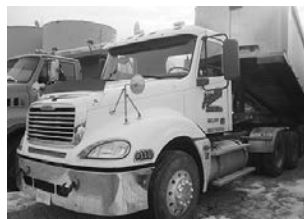
'10 FTL Columbia, DD15, 550 hp, 18 spd., 46R, wet kit, $49,500.
