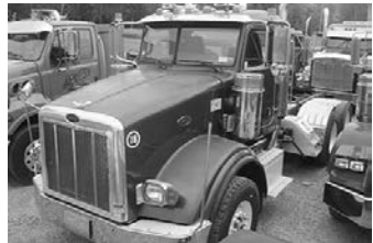
'06 Pete 357, 550 Cat, 8LL, Hend. susp., 20F, 46R, dbl. frame, 69,000 ORIGINAL MILES, air ride avail., $76,000.
