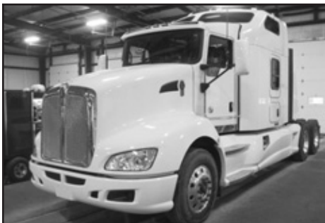
'12 KWT660 , 72" slpr., ISX 500 hp, 10 spd., 3.36 ratio, loaded, bunk beds, fridge.
