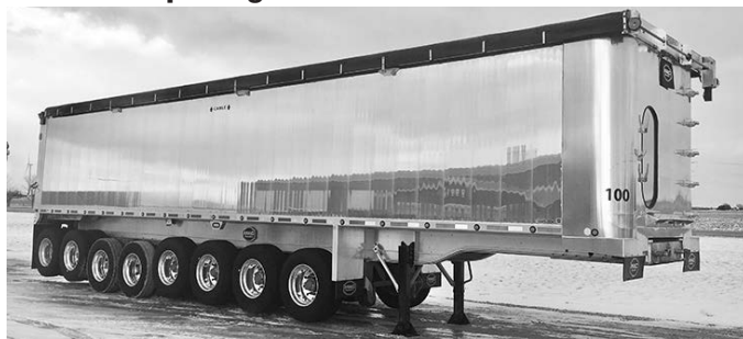
Used '19 MAC 8-axle dump, 43'x102', 84" side, disc brakes, Michelins, Durabrite whls., liner, frt. to back Cramaro elec. tarp, man door, call for pricing.
