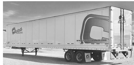
'11 Wabash van trlr., 53'x102', air ride, drum brakes, air sld., Hend. susp., S.S. rear frame & doors, S.S. frt. apron, food grade trlr., Hend. tire Mac Pro, virgin Michelin X Ones, $19,500.
