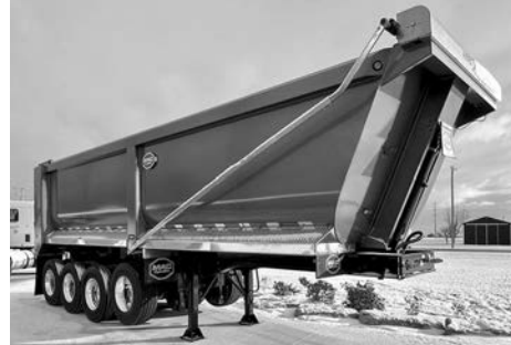
'24 MAC, Hardox AR450, 28' long, 96" wide, 66" tall, elec. tarp, 11R22.5 tires, drum brakes, air assist high liftgate, spg. ride, (1) left, color: gray, call for pricing.
