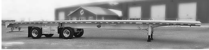
'18 MAC 53' flatbed , high spec'd, super singles, disc brakes, Durabrites, tire inflation.
