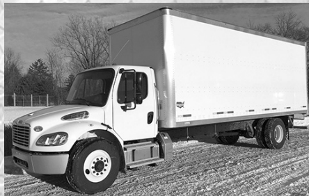
M2106 , 230 hp Det., Allison trans., 270" WB, 26,000 GVW, 24'x102"x102" Wabash body, $79,950 + tax & title.
