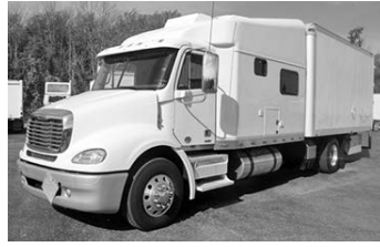
#6873 - '09 FTL Columbia 112, 130" RR splr., 430 hp Cat, Ultrashift 10 spd., 12F, 23R, 18'x102"x103" Morgan van, $56,900.
