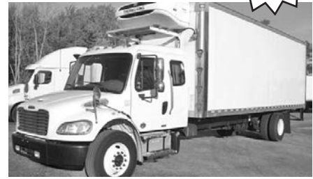
#7128 - '12 FTL M2 106, 28" ext. cab, 250 hp Cum., auto., 33,000 GVW, 26'x102"x103" Morgan van, TK reefer unit, $33,900.
