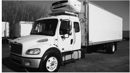
#6894 - (2) 14 FTL M2-106, 28" ext. cab, 250 hp Cum., 6 spd., air ride, 12F, 21R, 26'x102"x97" Morgan reefer, $51,900.
