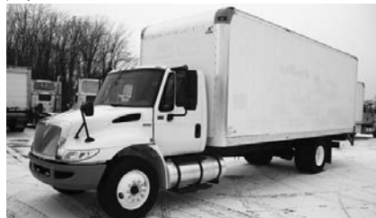
#6973 - '12 Int'l. 4300, 230 hp, DT466, auto., 25,999 GVW, under CDL, 24'x102"x97" Supreme van, Maxon liftgate, $23,900.
