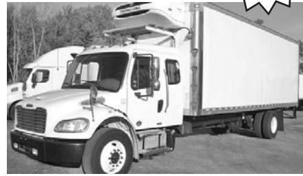
#7128 - (3) '12 FTL M2 106, 28" ext. cab, 250 hp Cum., auto., 33,000 GVW, 26'x102"x103" Morgan van, TK reefer unit, $33,900.
