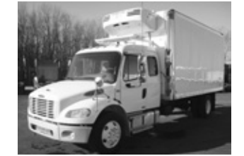
#5227 - '06 FTL M2, 28" slpr., 250 hp Cat, auto., 26,000 GVW, under CDL, 18'x102"x103" Morgan reefer, R.U., $34,900.
