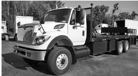
#6859 - '09 Int'l. Work Star, 370 hp Cum., 10 spd., 18F, 40R, 26'x102" Ledwell & Sons flatbed, dbl. frame, MaxLift boom, $55,900.
