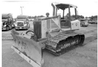
'13 Deere 700K LGP, OROPS, new U/C, pads @ 60%, strong running machine, tight 6-way blade, 50% cutting edge, hystat variable spd. . . . . $69,500
