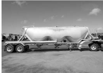
'04 Heil bulk trlr., 70,000# GVWR, alum. frame, air ride susp., air brakes, alum. tank, 3-compt., 295/75R22.5 tires, 1040 cu. ft., #23D1221A . . . . . $26,500
