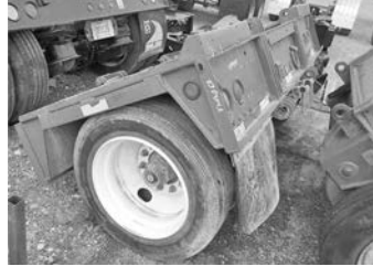
'93 Trail King Booster, Trail King pin on axle pin through axle, 2300 lbs., 5", S/A, call for more details, #23D404A . . . $6,000
