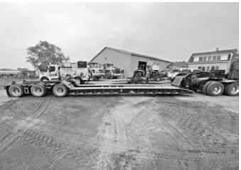
'20 Fontaine 55HFLD, 132,332# GVWR, air ride susp., air brakes, hyd. gooseneck, 26' main deck, boom recess, Honda gas powered self-contained hyd. system, alum. whls., 275/70R22.5 tires, #23C8075 . . . . . $114,500
