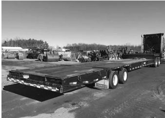
'17 Pitts HD35 hyd. tail, 87,900 GVWR, 50' overall length, 102" overall width, 10'9" frt. deck, 31'9" main deck, 8'6" rear deck, air brakes, air susp. .... $39,500
