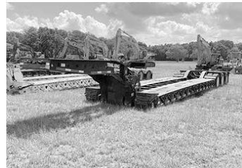
'16 Trail King TK10HDG, tri-axle, air ride, 3rd axle lift, set up for 4th axle, steel whls., pilot hubs, 26'x102" well, outriggers, D-rings, pony motor, 2 pin pace neck, #22E5034 . . . . . $89,500
