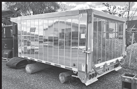
New East Genesis 2, 11.5'x102"x60", 3-way air gate, pre-wired for tarp, tail lights, marker lights, strobe lights already installed, $20,000.
