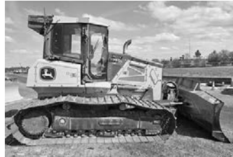
'21 Deere 750L LGP, 6-way blade, EROPS, A/C, heat, sweeps, rear screen, rear hyd., wide pads, U/C like new, ready to go to work, 7056 hrs., stk. #9153 . . . $129,500
