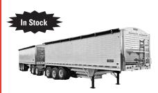
New Wilson 8-axle alum. break-up hopper trains, 28'6"x102"x78" side ht., air ride tri-axles w/frt. lift and a NEW Wilson air ride dolly, 1900-Bu. legal!
