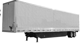
New 2021 Utility 4000-DX Composite Wall Vans, 100" I.W., Hend. Ultraa-K susp., Hend. Tiremaax Pro infl. H.D. 16" & 24" O.C. logistic posts, snag-free foam core walls, 20K forklift rating, S.S. rear frame, only 13,200 lbs.!
