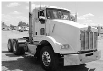
'14 KWT800, 492,330 miles, Cum. ISX 12, 330 hp, FRO14210C trans., 12F, 40R, 170" WB, air ride susp., #104581, $44,900.
