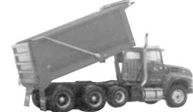
Tri-axle dump truck, set up w/rock boxes.
