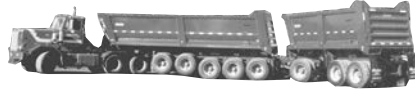
Rhodes 5/X & 6/W excavator, tare wt. 41,000, 54" sides, 1/4" AR400 throughout. Call us about features & specs, GVW 159,000.
