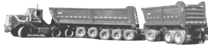
Rhodes 5/X & 6/W excavator, tare wt. 41,000, 54" sides, 1/4" AR400 throughout. Call us about features & specs, GVW 159,000.
