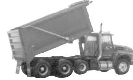
Tri-axle dump truck, set up w/rock boxes.
