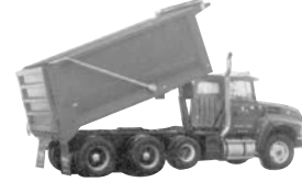
Tri-axle dump truck, set up w/rock boxes.
