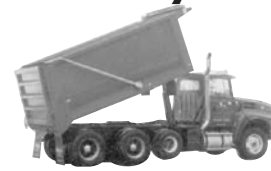
Tri-axle dump truck, set up w/rock boxes.
