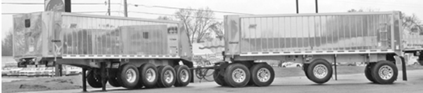
New East Genesis Super Train , alum. frame, alum. whls., 27,700 lbs.
