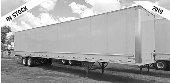
(50) New Stoughton 53' air ride, Z plate, exterior rub rails, PSI tire inflation system, corrugated steel roof, hard plastic scuff.
