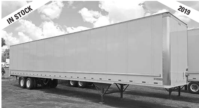
(7) New Stoughton 53' air ride Z-plates , exterior rub rails, PSI tire inflation system, corrugated steel roof, hard plastic scuff.
