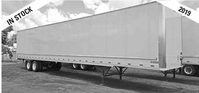
(50) New Stoughton 53' air ride Z plate , exterior rub rails, PSI tire inflation system, corrugated steel roof, hard plastic scuff.
