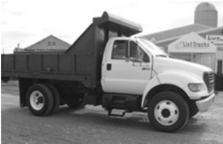
'03 Ford F750 dump , Cat 3126, push button auto., 30,000 GVW, air brakes, 12' dump w/24" sides, tarp, 134,000 miles, pintle hook & elec. brakes in rear, stk. #630.
