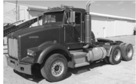
'95 KWT800, Cat 3406, 455 hp, 10 spd., 12F, 46R, wet kit, 402,000 miles, dual exh., (6) alum. whls., stk. #632.
