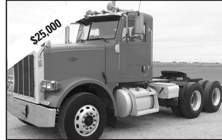
'06 Pete 378 , Cum. ISX, 400 hp, 10 spd., 12F, 40R, air ride, 3.70 ratio, alum. whls., visor & tanks, sharp looking truck, stk. #1595.
