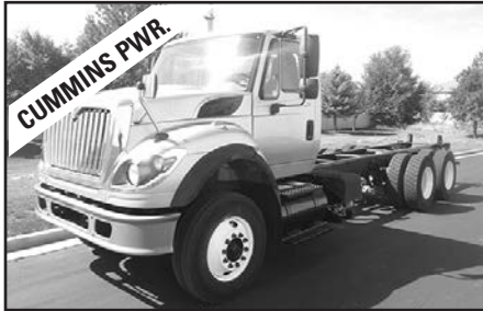
'10 Int'l. 7600 tdms. , Cum. ISM, auto., 14F, 40R, 24' of frame, 250,000 miles, lease maintained, will upfit to your needs, stk #7600.
