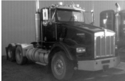
'96/'97 KW T800 Michigan Special, Cat 3406, 475 hp, 18F, 46R, quad lock, wet kit, '97 has 13 spd. w/492,000 miles, '96 has 18 spd. w/660,000 miles & o'haul, dual exh., alum. whls., stk. #631.
