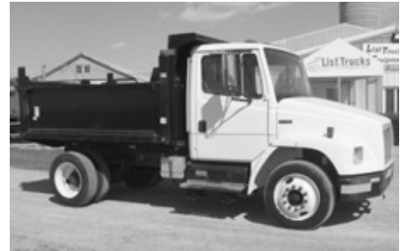
'00 FTL FL70 dump , Cat 3126, 230 hp, 6 spd., under CDL, 220,000 miles, new 10' dump w/fold down sides, good rubber, clean truck, stk. #590.
