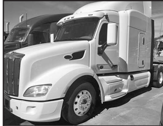
'15 Pete 579 , Cum. ISX15, 450 hp, 10 spd., Pete Low Air Leaf susp., 3.25 ratio, 22.5 LP, alum. whls., 239" WB, 12F, 40R, 72" raised roof slpr., stk. #UFD258969-UFD258978.
