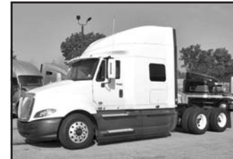
'11 Int'l. Prostar, Cum. ISX15, 435 hp, 10 spd., air ride susp., 2.64 ratio, 22.5 LP, 230" WB, 12F, 40R, 72" raised roof slpr., stk. #UBN372492.
