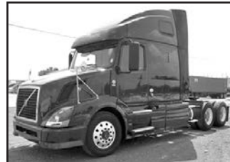
'12 Volvo VNL64T670, Cum. ISX15, 450 hp, 10 spd., air ride, 3.42 ratio, 22.5 LP, alum. whls., 217" WB, 12F, 40R, 61" raised roof slpr., stk. #UCN535918.
