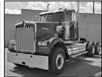
'18 KW W900L, Cum. X15 1850 lb. ft., 565 hp, 18 spd., AG 460 susp., 3.91 ratio, Goodyear 385/65R22.5-18 frt., Michelin 11R22.5-16 rear, 209" WB, 20F, 40R, stk. #JJ194319.
