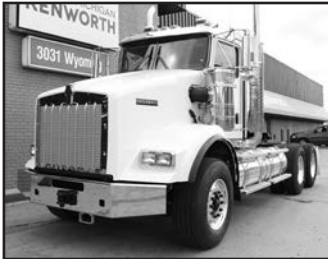
'18 KW T800, Cum. X15, 565 hp, dsl., tdm., 18 spd. O.D., eng. brake, 3.91 ratio, 385/65R22.5 Goodyear frt. tires, 11R22.5 Michelin rear tires, 195" WB, stk. #JJ203153.
