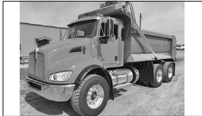
'18 KW T370, Paccar PX9, 350 hp, Hend. PRIMAAX susp., 5.57 ratio, 22.5 std., 184" WB, 16F, 40R, stk. #JM216719.
