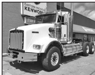
'18 KWT800, Cum. ISX 1850 lb. ft., 565 hp, 18 spd., Ag 460 susp., 3.91 ratio, Goodyear 385/65R22.5-18 frt., 11R22.5-14 rear, 195" WB, 20F, 46R, stk. #JJ199913.
