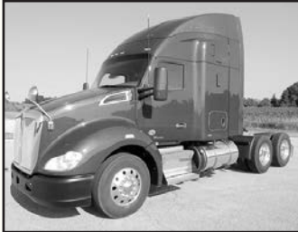
'15 KWT680 , Paccar MX13, 455 hp, 10 spd., AG 380 susp., 3.07 ratio, 22.5 LP, 200" WB, 12F, 40R, 52" mid-roof slpr., stk. #UFJ435974.
