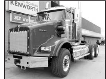
'18 KWT800, Cum. X15 1850 lb. ft., 565 hp, 18 spd., Ag 460 susp., 3.91 ratio, 385/65R22.5 Goodyear frt., 11R22.5 Michelin rear, 195" WB, 20F, 46R, stk. #JJ203159.
