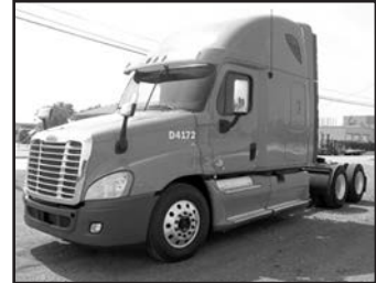
'12 FTL Cascadia 125 , Det. DD15, 475 hp, 10 spd., air ride, 3.31 ratio, 22.5 LP, alum. whls., 230" WB, 12F, 40R, 72" raised roof slpr., stk. #UCSBL6652.
