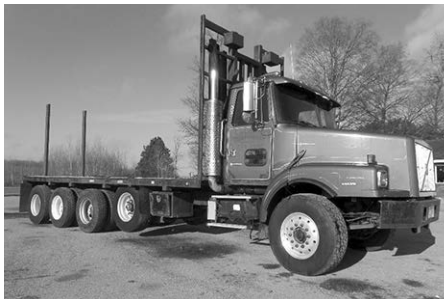
'97 Volvo 5-axle log truck, M11 Cum., 350/400 hp, 10 spd., 24' log bed w/fish-mouth hitch, $19,500.
