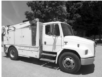
'00 FTL FL70 service truck, ISB Cum., 225 hp, Allison auto., 13' mechanic's body w/toolboxes, model 6006H Autocrane, welder/gen., aux. fuel tank, $37,500.
