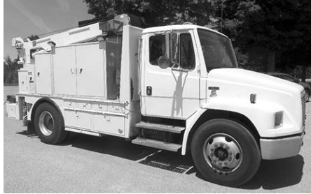
'00 FTL FL70 service truck, ISB Cum., 225 hp, Allison auto., 13' mechanic's body w/toolboxes, model 6006H Autocrane, welder/gen., aux. fuel tank, $37,500.
