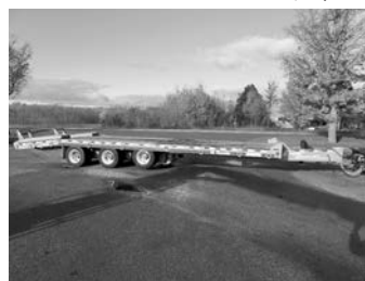
New Eager Beaver 25-ton tag-along, tri-axle w/lift axle, spg. ride, $26,900 + taxes. (3) Other Eager Beaver trailers in stock.
