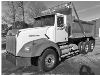
'05 Western Star tdm. dump, 375/430 Det. Dsl., 10 spd., 12F, 40R, w/new 14' demo body, Roll-Rite tarp systems, 45-ton hitch.
