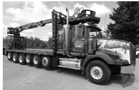
'06 Western Star 7-axle log truck, C15 Cat, 475 hp, 8LL, 20F, 46R, air ride, w/Serco 8500 ldr., approx. 150,000 miles on Cat Platinum eng. o'haul, recent trans. & frt. diff.
