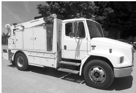
'00 FTL FL70 service truck, ISB Cum., 225 hp, Allison auto., 13' mechanic's body w/toolboxes, model 6006H Autocrane, welder/gen., aux. fuel tank, $37,500.
