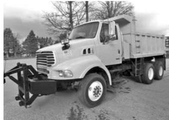
'02 Sterling tdm. dump, 3126 Cat, 300 hp, Allison auto., 12' box, underbody blade, frt. plow mount, pintle hitch, $24,900.
