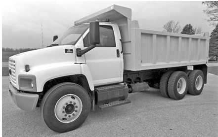
'07 Chevy C8500 tdm. dump, 7.8L, 275 hp, Allison auto., Hend. susp., 14F, 40R, steel pilot whls., 11R22.5 tires, new 15' dump box, $57,500.
