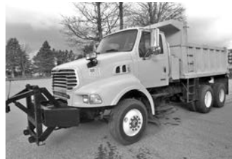
'02 Sterling tdm. dump, 3126 Cat, 300 hp, Allison auto., 12' box, underbody blade, frt. plow mount, pintle hitch, $26,900.
