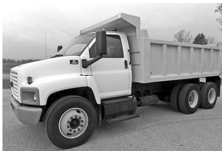
'07 Chevy C8500 tdm. dump, 7.8L, 275 hp, Allison auto., Hend. susp., 14F, 40R, steel pilot whls., 11R22.5 tires, new 15' dump box, $59,500.
