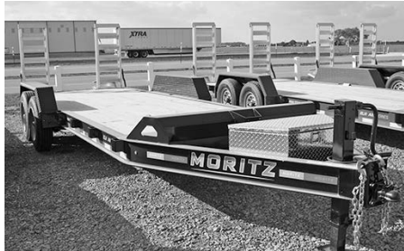
'22 Moritz 7'x20' H.D. equipment trlr. , bumper pull 2-axle, alum. ramps, 16,000# GVW, LED lights, elec. brakes, spare tire mount, $11,550.
