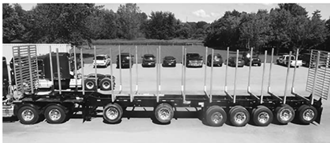
'19 Pratt 7-axle logging trlr., 53'x102" air ride, alum. hubs & whls. on super singles, frt. 2 & rear 3 lift w/manual dump valve, alum. deck, alum. stakes, alum. frt. & rear gates, F.O.B. Gaylord, MI. Due in mid-October. Call for more information.
