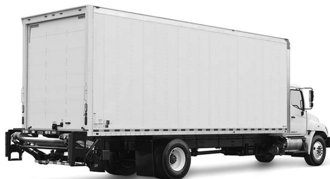
NEW '18 Morgan 24' or 26'x103"x102" GVSD alum. dry freight van body, full plywood lining, Hi-Lo pkg. (includes 24" threshold plate, (4) extra CMs at rear, reinforced frt. end, & 12" scuff), translucent roof, (2) rows of E-track, 10" dock, ICC bumper. Fast track body from Morgan in 2-4 weeks. Call for more details.
