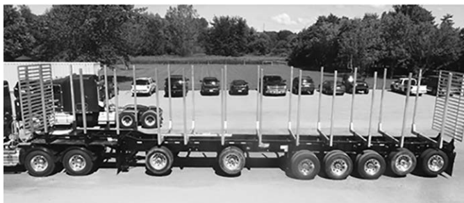
'19 Pratt 7-axle logging trlr., 53'x102" air ride, alum. hubs & whls. on super singles, frt. 2 & rear 3 lift w/manual dump valve, alum. deck, alum. stakes, alum. frt. & rear gates, F.O.B. Gaylord, MI. Due in early August. Call for more information.
