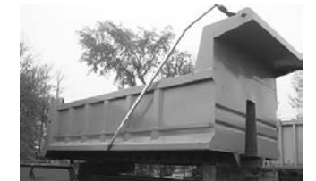
New steel dump box, w/tarp.
