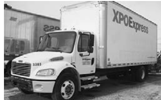
'04 FTL M2, dsl., auto., non-CDL, air brakes, Morgan van body.
