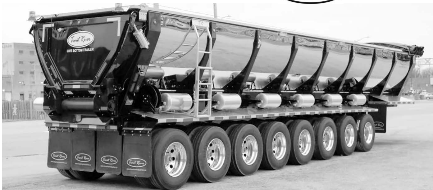
NEW TROUT RIVER LIVE BOTTOM, 8-AXLE, (4) LIFT AXLES, AIR DISC BRAKES, TIRE INFLATION SYSTEM, ALUMINUM WHEELS, 51-52 TON CAPACITY.
