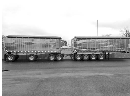
2019 East Genesis Super Train 28.5' lead, 25' pup, 102" wide, 76" sides, alum. frame, air ride, (2) lifts on lead, June delivery.
