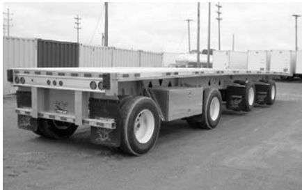
Manac 48' Steel 4-Axle All galvanized w/wood deck, (2) lift axles, (2) alum. tool boxes. Available for rental.
