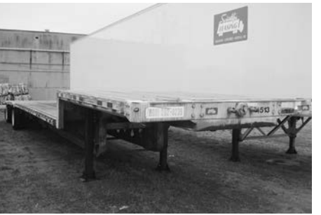
2015 Manac 48'x102" Combo Flatbed Steel frame, alum. deck, alum. crossbars, alum. side rails, very nice trlr., $21,500.
