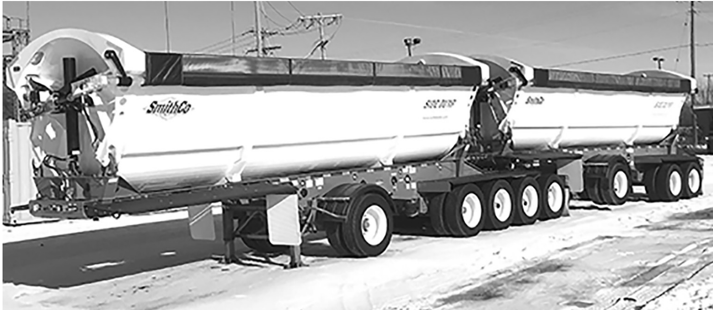
2018 SMITHCO SIDE DUMP, 65-YD. CAPACITY, B-TRAIN CONFIGURATION, MICHIGAN STYLE TUBS, AR400, 102" WIDE, DUAL CYLS., DUMPS TO EITHER SIDE, AIR RIDE SUSP., IN STOCK NOW.
