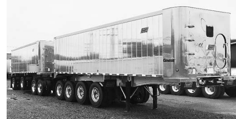
2019 East Genesis Super Train 28.5' lead, 25' pup, 102" wide, 76" sides, alum. frame, air ride, (2) lifts on lead, elec. water tight tarps, in stock.
