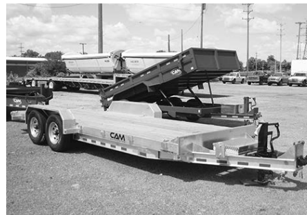
2019 CAM SuperLine Galvanized 7-Ton Equipment Hauler All galvanized frame, tongue, fenders & whls., 102" wide, 20'x81" deck, payload of 12,900#, $10,500.
