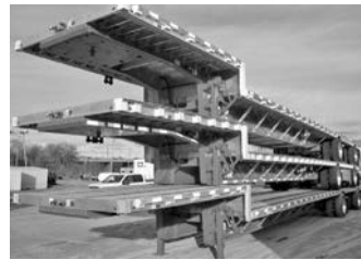
2024 Wilson Combo Drop Deck 53'x102" 10'1" Air ride spread, all alum. whls., (2) tool boxes, S.S. doors, winch track both sides, H.D. side rails w/dbl. spools.
