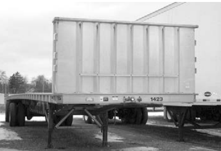
2012 Wilson Combo Flat 48'x102" Steel main beams, alum. deck, 10'1" spread, air ride, $19,900.
