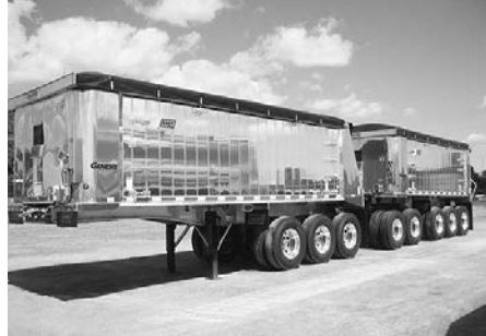
2019 East Genesis Triple Ten Train 24-1/2' Lead, 19' pup, air ride susp., alum. whls., alum. frame, Rollrite electric cable style tarp system, HMW floor liner, in stock.
