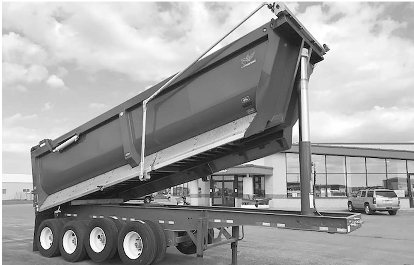
NEW 2018 MANAC QUAD-AXLE DUMP, (1) OR (2) LIFT AXLES, 1/4" AR450 HARDOX STEEL FLOOR, SIDES BULKHEAD & TAILGATE, REYCO 21B TRI-AXLE (REAR), ROLL-RITE KNUCKLE ARM TARP, BOTH STD. TAILGATE & HIGH LIFT TAILGATE MODEL ALSO AVAILABLE, IN STOCK NOW.
