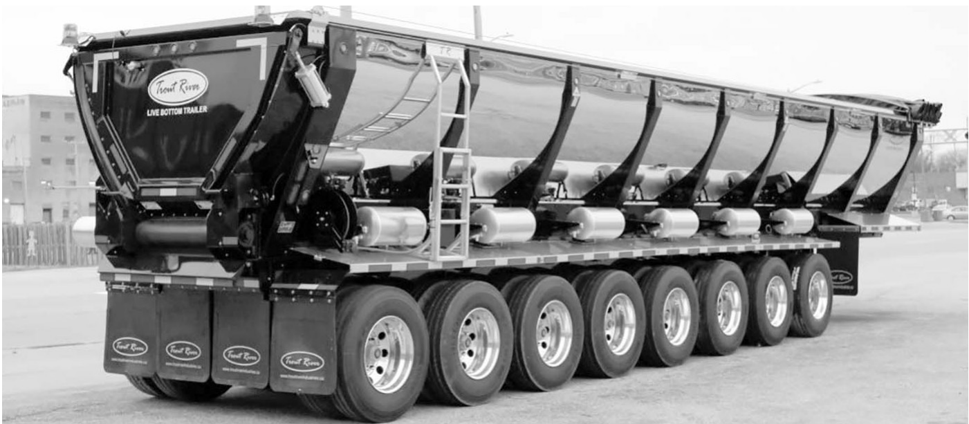
NEW TROUT RIVER LIVE BOTTOM, 8-AXLE, (4) LIFT AXLES, AIR DISC BRAKES, TIRE INFLATION SYSTEM, ALUMINUM WHEELS, 51-52 TON CAPACITY.
