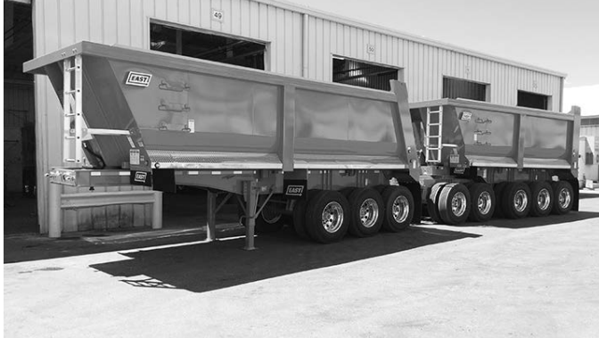
2021 East AR450 Steel Triple Ten Train 24' Lead, 19' pup, AR450 Hardox steel, 60" tailgates w/ext. hinges, all alum. whls., Reyco 21B spg. ride, ladders upon request, May delivery.
