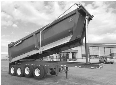
New 2019 Manac Quad-Axle Dump AR450 Hardox steel floor, sides, bulkhead & tailgate, Reyco 21B tri-axle plus air lift, Roll-Rite knuckle arm elec. tarp system, highlift & std. tailgates.
