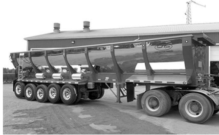
40-Ton Live Bottom All air ride w/(3) lift axles, drum & shoe brakes, alum. whls., Cramaro elec. asphalt tarp system.
