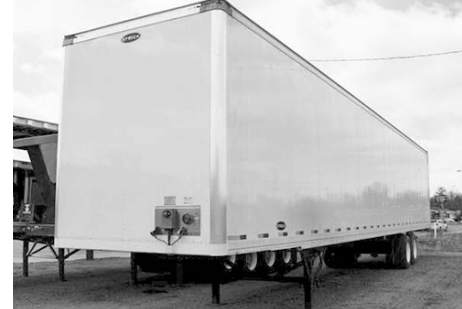
2018 Strick 53'x102" TFI Air Ride Van Alum. sheet & post w/snap-in HDPE int. lining, 12" galv. roof, galv. spg. tension roof bows, H.D. frt. wall w/(5) upright posts & int. lining @ 1/2", structure wood & 12" steel scuff @ btm., composite rear swg. doors.
