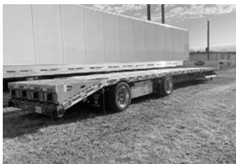
Used 2023 Wilson 53' Drop Deck w/Beavertail, (2) tool boxes, ramps for upper deck, (4) flip-over ramps at rear.
