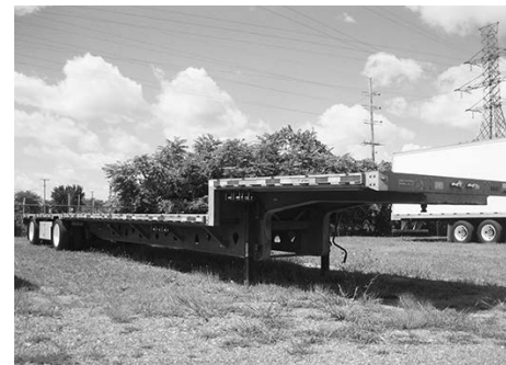
2013 Manac 53'x102" Galv. steel drop deck , hot dip main beams, CM's, side rails, rear bumper, wood plank floor, winch track, winches, air ride, 60" alum. toolbox, #1441, $25,000.
