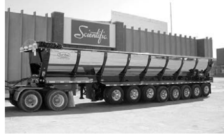
50-Ton Live Bottom Live bottom, air ride w/(4) lifts, drum brakes, alum whls., elec. Cramaro tarp system, coming in April.
