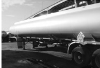
(3) '08 Heil 9500-gal., 4-compt., alum., D/H, air ride, alum. whls., wide base tires.
