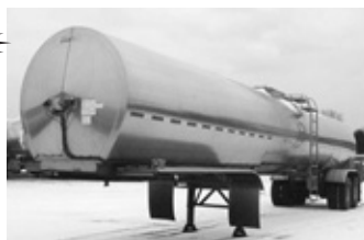
(3) '03/'04 Brenner, 7500-gal., 3-compt., all S.S. frames to hangers, air ride, 22.5 steel disc whls., 2-1/2" pump.
