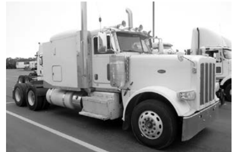
'12 Pete 388, Cum. ISX, 500 hp, 18 spd. manual, 60" flat top slpr., 14.6F, 46R, 4-whl. locks, chrome dual exhaust & breathers, stk. #Y24172.
