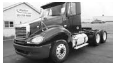
#3273 - '07 Columbia, 531,000 miles, 14L Det., 455 hp, 12F, 40R, air ride, 10 spd., 3.73 ratio, 169" WB, Ryder maintained, $32,000.
