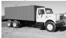
#3271 - '00 Int'l. 4900, 86,592 miles, DT466, 225 hp, new brakes & drums, 14.6F, 40R, Hend. beam, Allison auto. 653, 5.38 ratio, 156" C.T., 18" used box, frt. post hoist, from Tennessee, no rust, call.
