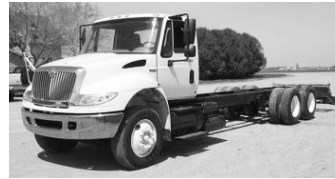
#3268 - '09 Int'l. 4400, DT466, 260 hp, 12F, 40R, air ride, Allison auto. XMSN 3000HS, 5.29 ratio, 272" WB, A/C & cruise, $32,000.
