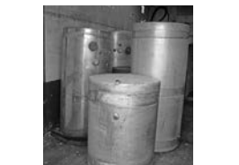
Aluminum & steel fuel tanks.
