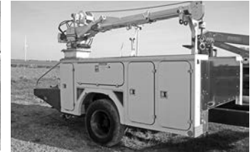
#3253A - 11' Fiberglass service body, 10' reach Pitman, HY crane & winch, 12-volt-110 elec. converters, HY legs on back for crane, winch cap. 25,000 lbs. to 7000 lbs.
