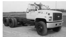
#3285 - '99 Chevy C8500, only 79,214 miles, Cat 3126 230 hp, brakes like new, 11x22.5 drives 80%, steering 80%, L40%, R75%, 14.6F, 34R Hend. beam, Allison auto 653 PTO gear, 4.33 ratio, CT 124, 15' frame, pin-tie hitch, air lines to back for trlr. brakes, driver's seat air ride, seats (3) people, $14,500.
