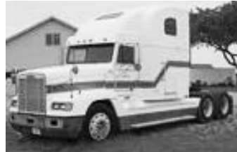
#2024 - '01 FTL FLD120, 12.7 Det., 430 hp, Super 10M spd., 12F, 40R, new A/C, cruise, Jake.
