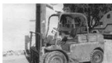
#Hyster Fork Lift - '69 Hyster H80C, 6-cyl. Continental F227, 3 spd. w/forward & rev., 12,150#, 46" forks, 6% back tilt, 8500# max. load at 18", 14' lift ht.
