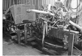
(2) Engine cores, C10 Cat & Cat 3126, 300 hp.
