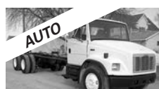
#3200 - '03 FTL FL80, 231,000 miles, Cat 3126, 250 hp, Allison auto., 14F, 40R, air ride, 5.29 ratio, 25' of dbl. frame, call.
