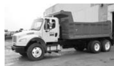
#3278 - '08 FTL M2, 341,000 miles, Cum. ISC, 330 hp, 16F, 315R22.5 frt. @ 75%, 40R, air ride, FROF12210C 10 spd., 4.33 ratio, new American 15" gravel box, all hi-tensile steel, 3/16 floor, 1-pc. 50,000 PSI, 44" sides, Ryder maintained, call.
