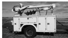
#3253A - 11' Fiberglass service body, 10' reach Pltman, HY crane & winch, 12-volt-110 elec. converters, HY legs on back for crane, winch cap. 25000 lbs. to 7000 lbs., $5,500.
