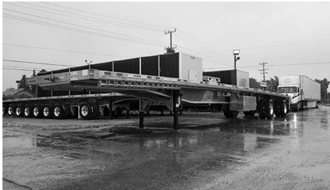
New 2020 Manac Darkwing, 53', all alum. flatbed, rear sldg. axle, tool box, Apitong wood nailers, General 11R22.5 tires.
