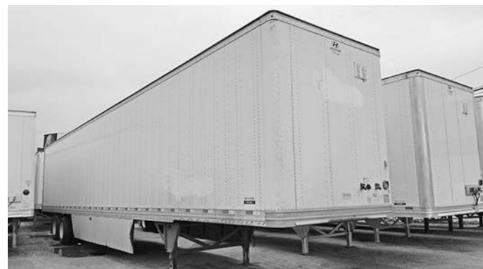
(4) 2016 Hyundai vans, 53', air ride, swing door, skirts, tire inflation, vents, air assist pin release
