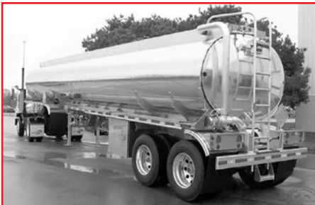
(2) 2025 LBT 42' tanker MC406 , 9200-gal., 1-compt., disc brakes, super single tires, w/roll stability, $114,563 ea.
