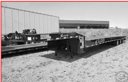
2025 XL Specialized 110 sliding axle drop deck , 53', 55-ton/110K lb. cap., sliding tri-axle, trailer tilts creating a ramp, $140,811.
