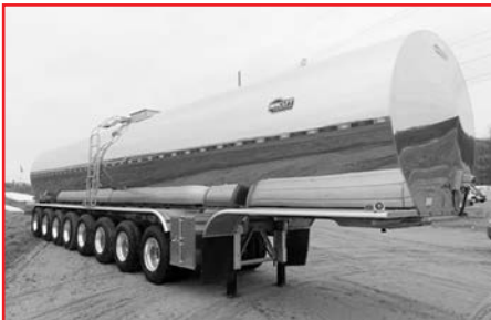
2024 MAC LTT 49' sanitary tanker , 8-axle, 12,200-gal., (5) lifts, 1-compt., tire inflation system, call for price.
