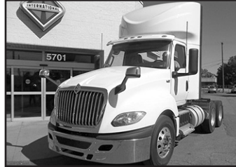
'18 Int'l. LT625 6x4 day cab tractor, Cum. ISX 15L dsl., 450 hp, 450 hp, Fuller 10 spd. trans., conventional cab w/Deluxe int., air ride susp., air brakes, eng. brake, A/C, PS, 52,350 GVW, 12.35F, 40R, 177" WB, 3.42 ratio, disc steel whls., 11R22.5 tires, air slide 5th whl., 160-gal. (80+80) dsl. fuel cap., stk. #NTJN445610, call for price!
