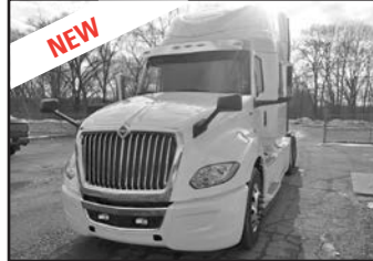
'19 Int'l. LT625 SBA 6x4 slpr. tractor w/73" Hi-Rise & Cum. X15 dsl., 450 hp, Fuller 10 spd. automated manual trans., conventional cab w/1 bunk & Diamond int., refrigerant, air ride susp., air brakes, eng. brake, PS, A/C, 52,350 GVW, 12.35F, 40R, 228" WB, 2.64 rear end ratio, polished alum. whls., 22.5" tires, 220-gal. (120+100) dsl. fuel cap., stk. #NTKN501385, call for price!
