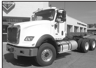
'18 Int'l. HX620 6x4 day cab tractor, Cum. X15 dsl., 565 hp, Fuller 18 spd. trans., conventional cab w/Deluxe int., Hend. susp., air brakes, eng. brake, PS, A/C, 64,000 GVW, 18F, 46R, 191" WB, 3.91 ratio, disc whls., 11R22.5 tires, air slide 5th whl., 150-gal. dsl. fuel cap., stk. #NTJN568102, call for price!
