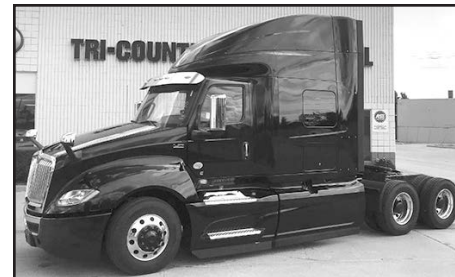
'19 Int'l. LT625 6x4 slpr. tractor, 73" hi-rise, Cum. X15 dsl., 500 hp, Eaton 12 spd. auto., Eaton Endurant 12 spd. fully automated manual, conv. cab, Diamond int., dbl. bunk, refriger., air ride susp., air brakes, eng. brake, PS, AC, 52,350 GVW, 12.35F, 40R, 228" WB, 2.79 ratio, pol. alum. whls., 22.5x8.25 tires, air sld. 5th, 240-gal. (120+120) dsl. fuel tank, stk. #NTKN313912, call for price!
