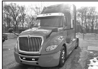
'19 Int'l. LT625 6x4 dbl. bunk slpr. tractor w/73" Hi-Rise & Cum. X15 dsl., 500 hp, Fuller 13 spd. trans. w/dbl. O.D., conventional cab w/Diamond int., refrigerant, air ride susp., air brakes, eng. brake, PS, A/C, 52,350 GVW, 12.35F, 40R, 228" WB, 3.36 rear end ratio, air slide 5th whl., polished alum. whls., 11R22.5" tires, 220-gal. (120+100) dsl. fuel cap., stk. #NTKN501563, call for price!
