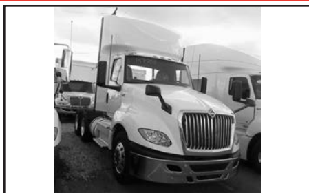
2019 Int'l. LT625 6x4 Day Cab Tractor, Cum. X15 dsl. w/430 hp, Eaton Endurant 12 spd. fully auto. trans., Conventional cab w/ Classic int., air ride susp., air brakes, eng. brake, PS, A/C, 52,350 GVW, 12.35F, 40R, 173" WB, 2.79 rear end ratio, polished alum. whls., 22.5x8.25 tires, air slide 5th whl., 140-gal. (70 + 70) dsl. fuel cap., Stk # NTKL566174 Call For Price!
