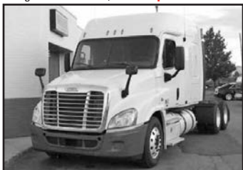
'11 FTL Cascadia tdm. axle 6x4 slpr. tractor w/70" mid-roof XT, Det. Dsl. DD15, 455 hp, 10 spd., conv. cab w/Benchmark int., dual bunks, dual high-back seats, air ride pass. seat, air ride susp., air brakes, eng. brake, A/C, PS, 52,000 GVW, 12F 40R, 240" WB, 3.55 ratio, alum. firt. whls., alum. outer rear whls., 22.5 tires, air slid. 5th whl., call for price.
