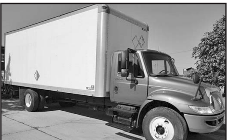
'12 Int'l. 4300 SBA 4x2 dry van w/24' Morgan body, Int'l. MaxxFace DT dsl. w/230 hp, Allison 5 spd. auto. w/O.D., conventional cab w/Deluxe int., wood floor, R.U. rear access door, liftgate, spg. susp., air brakes, PS, A/C, 25,999 GVW, 10F, 19R, 254" WB, 5.57 ratio, steel whls., 22.5" tires, 100-gal. alum. dsl. fuel tank, stk. #UTCH118879, $21,500.
