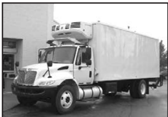
'10 Int'l. 4300 SBA 4x2 reefer truck w/TK TS-500 reefer unit & 22' Johnson FRP body, Int'l. DT466 dsl., 255 hp, Eaton Ultrashift, conv. cab w/deluxe int., R.U. rear access door, alum. floor, liftgate, spg. susp., air brakes, eng. brake, A/C, PS, 33,000 GVW, 12F, 21R, 238" WB, 4.88 ratio, steel whls., 11R22.5 tires, 100-gal. dsl. fuel tank, stk. #UTAH167039, call for price!
