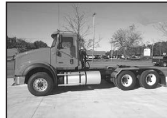
'18 Int'l. HX620 6x4 day cab tractor, Cum. X15 dsl., 565 hp, Fuller 18 spd. trans., conventional cab w/Deluxe int., air ride susp., air brakes, eng. brake, PS, A/C, 64,000 GVW, 18F, 46R, 191" WB, 3.91 ratio, disc whls., 11R22.5 tires, air slide 5th whl., 150-gal. dsl. fuel cap., stk. #NTJN568103, call for price!
