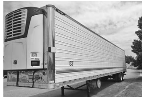
(10+) 2013 Great Dane 53'x102" flat floor reefers , logistic post, Carrier units, air ride slide suspension, stainless steel swing doors and rear frame.
