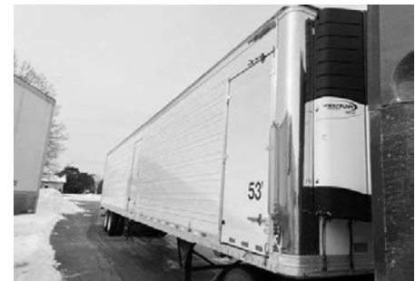
2010 Great Dane 50' & 53' , Carrier multi-temp units, duct floor, swing doors, air ride slide suspension, (2) curbside doors.
