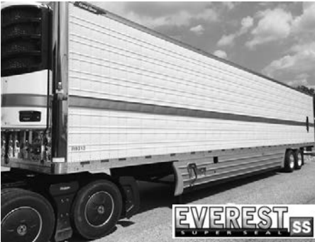
NEW 53'x102", duct floor, sliding tandem, stainless steel rear frame & doors, Hendrickson Ultra K, 40,000 suspension, laydon composite skirts, Thermo King Precident S700 unit.
