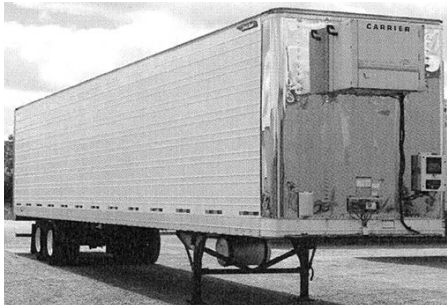
(10+) 2013 Great Dane 53'x102" dry vans , insulated w/Carrier heater units, stainless steel front, stainless steel doors, stainless steel rear frame & rear impact guard, air ride suspension, aluminum wheels.
