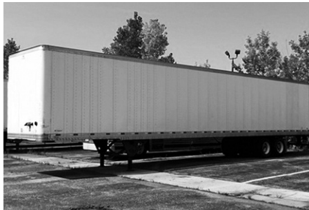
2013-2014 Hyundai sheet & post dry vans , 53'x102", logistic post on 24" centers, aluminum roof, swing doors, galvanized rear frames.
