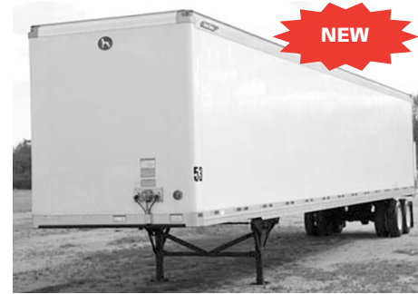
Coming in: 2020 Great Dane CS1 53'x102" dry vans, air ride, plastic lined interior, 16" center logistic posts, swing doors, aluminum roof.
