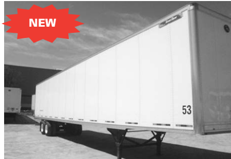
(10+) 2020 Great Dane Champion CP 53'x102" dry vans , air ride, tire inflation system, sliding tandem, 24" & 50" logistic posts, swing doors, aluminum roof.
