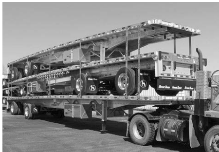
2020 Great Dane 53' all aluminum flatbeds , front fixed rear slide air ride suspension, aluminum deck w/(2) nailer boards, (2) tool boxes, (14) sliding winches w/straps, TireMaax Pro inflation system (Cowboy Edition).
