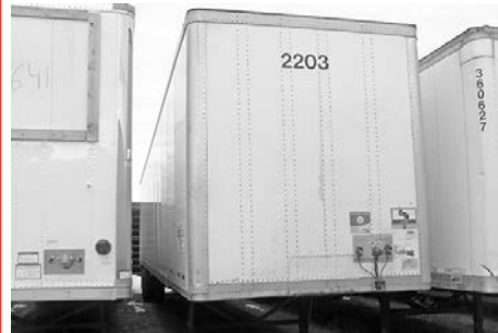
2004-2005 Wabash 53'x102" , spring ride, swing doors, aluminum roof, Duraplates.
