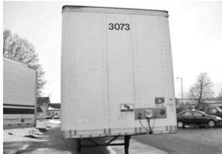
(3) '07 Wabash dry vans, 53'x102" , spg. ride, swg. doors, translucent roof, plywood lined, log post, 24" centers.
