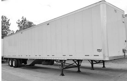
(3) 2014 Wabash Duraplates, 53'x102" , air ride slide, swing doors, aluminum roof, 24" logistics posts, sky lights, SmartTruck aerodynamics.
