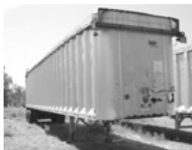
'05 Manac 48' alum. walking floor, 6" Keith slats, 102" wide, 91" ins., 13' ht., 11x22.5 Budd, Chalmers 46,000# susp., 80,000# GVW.
