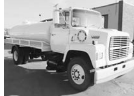
'88 Ford LT8000, spg. susp., 7.8L Ford eng., dsl., 11x22.5 tires, Allison auto., air brakes, 33,000 GVWR, 2000-gal. water tank, 137,116 miles, stk. #5955, $18,500.
