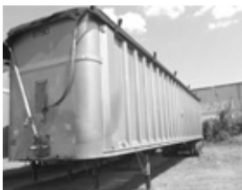
(3) '01 Steco, 45'x96", tdm., alum., walking floors, 105-yd. cap., tarp, 11x22.5 tires, located in Orlando, FL.
