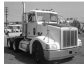
(2) '97 Pete 385 tdm. tractors, Cat 3306 dsl., 300 hp, 9 spd., A/C, 158" WB, 44R, air ride susp., 11x22.5 tires, 3.70 ratio, spoke whls., 375,000 miles.
