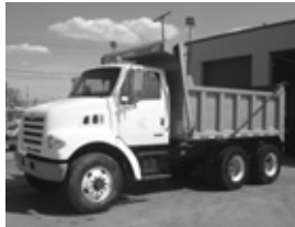
'04 Sterling LT7500 12' steel tdm. dump, tarp, pintle hitch, rear air hook up, Cum. 8.3L, 260 hp dsl., Allison MD3560 auto., A/C, 16F, 40R, dbl. frame, 26,000 act. miles.
