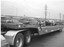
'97 Landoll 317, tdm., 35-ton cap., 48'x102", air ride susp., 20,000# winch, 10x17.5 tires, hub pilot, fork lift pkg., one-owner.
