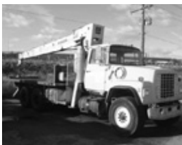
'85 Ford LT8000, tdm., 15-ton RO-Stieger crane, TC150-1, 64' tip ht., (4) hyd. outriggers, 20' flatbed, Cat 3208, 210 hp, dsl., Allison auto., 55,000# GVW, 207,000 miles, county owned!
