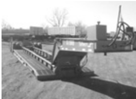
'92 Talbert tdm. 35-ton drop side, hyd. detachable lowboy, 24' well, 96" wide, 18" height, air ride susp., 255/70x22.5 tires.
