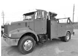
'97 Pete 330 service truck, Cum. 8.3, 9 spd. Eaton Fuller, 177" WB, 12-compt. service body, spool winch, stk. #CL 922, $32,500.
