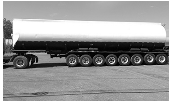
'74 Etnyre, steel tanker, steel sub-frame, 15,000-gal., 4-compt., 8-axle (4-down, 4-lift), newly refurbished, $24,000.
