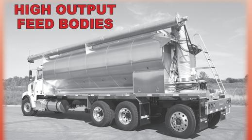
Unload up to 7000 lbs. per minute, 12-15-12 auger set up, many different configurations available, call for a quote.
