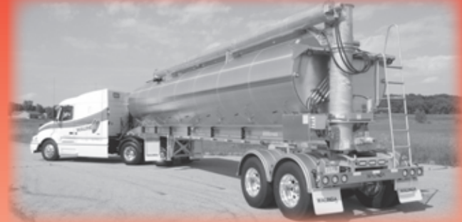
Unload up to 7000 lbs. per minute, 12-15-12 auger set up, many different configurations available, call for a quote.
