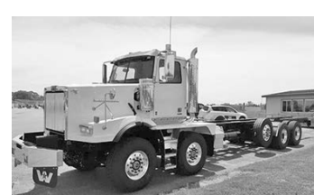
'20 Western Star 4900TS , Det. DD15, 14.8L, 400-505 hp, Allison 6 spd. auto., 109,500 GVWR, twin steer, #118424.
