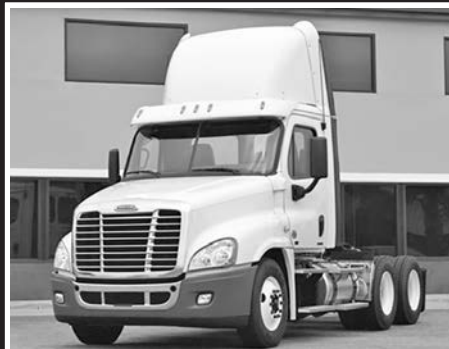
New '19 FTL Cascadia , 450 hp DD13 Detroit, DT12 trans., air ride, 3.23 ratio, 12F, 40R, eng. brakes, stk. #W19090.
