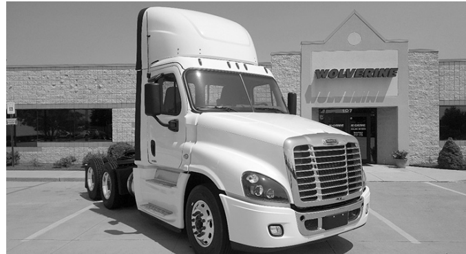
New '18 FTL Cascadia day cab, Evolution Aerodynamic pkg. , DD15, 400 hp, Det. D12 trans., 2.41 ratio, 52,000 GVW, air slide 5th, dual 80-gal. fuel tanks, alum. whls., stk. #W18023.
