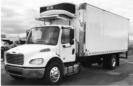
New '20 FTL M2 106 , B6.7 Cum., Allison auto., 220 hp, 234" WB, 26,000 GVW, stk. #D20014.
