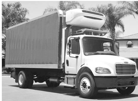
New '19 FTL M2-106, reefer, Det. DD5, 240 hp, Allison 2500HS auto., air ride, 26,000 GVW, stk. #W19146.
