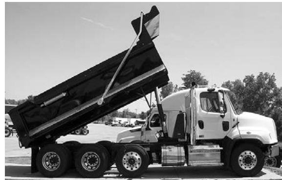
New '18 FTL 114SD tri-axle dump , DD13, 370 hp, 216" WB, 18F, 46R, 4.10 ratio, 77,200 GVW, Godwin dump body, stk. #W18024.
