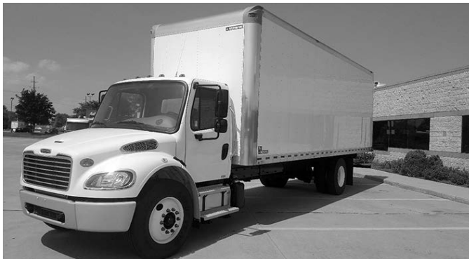
New '18 M2 106 van body , DD5, 230 hp, Allison auto, UNDER CDL , 26,000 GVW, air ride, 5.56 ratio, air brakes, 50-gal. fuel tank, 26' Morgan alum. van body, 103"x102" translucent roof, R.U. door, 12" dock ext., (2) rows E-Track, stk. #E18088.
